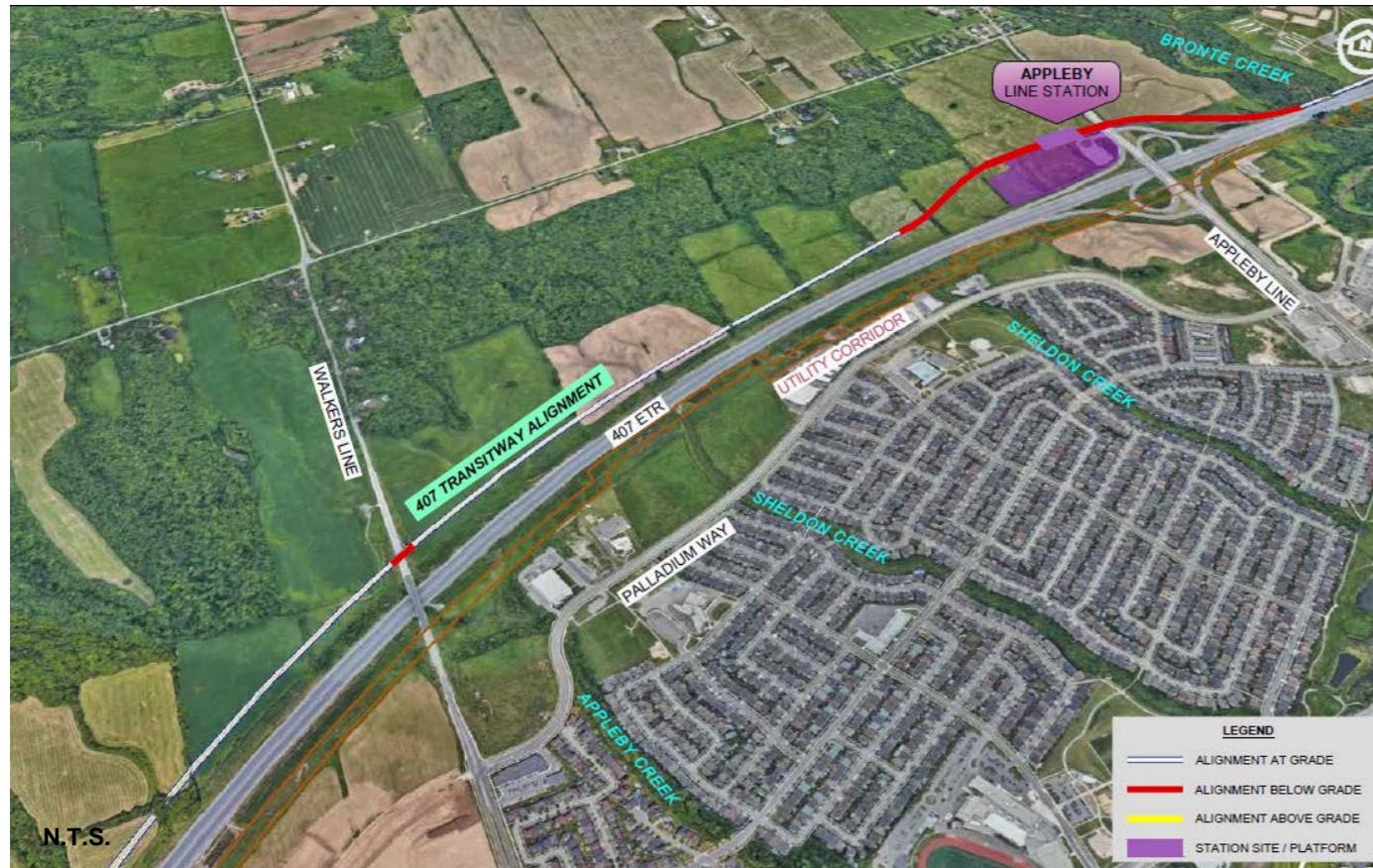
FIGURE 5.3: SEGMENT 2, EAST OF DUNDAS STREET TO EAST OF APPLEBY LINE ALIGNMENT LAYOUT.
