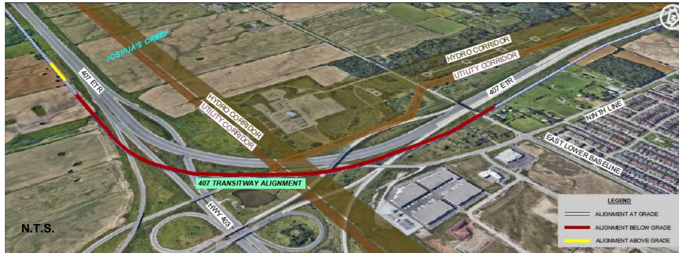
FIGURE 5.7: SEGMENT 6, EAST OF TRAFALGAR ROAD TO NORTH OF LOWER BASE LINE ALIGNMENT LAYOUT.
