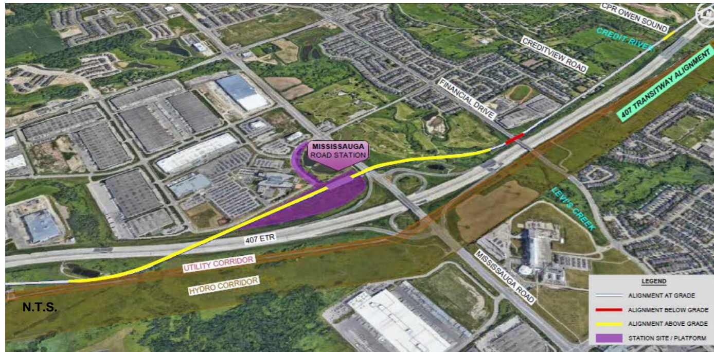
FIGURE 5.11: SEGMENT 10, WEST OF HERITAGE ROAD TO EAST OF CREDITVIEW ROAD ALIGNMENT LAYOUT.
