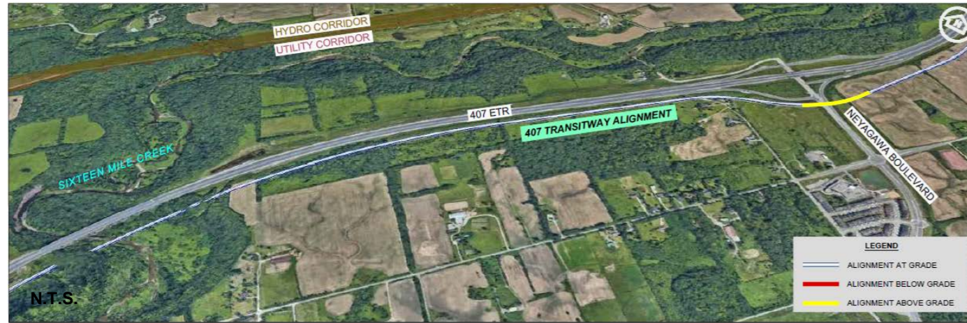
FIGURE 5.6: SEGMENT 5, WEST OF SIXTEEN MILE CREEK TO EAST OF TRAFALGAR ROAD ALIGNMENT LAYOUT.
